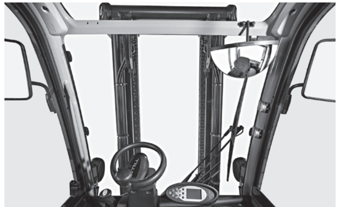
Narrow mast profiles for excellent visibility of forks and load at all times
