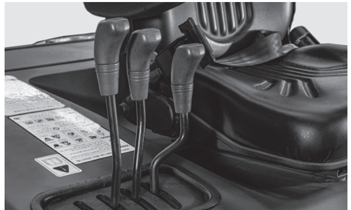
The multi-lever controls give the operator maximum control when using the hydraulic lifting system
