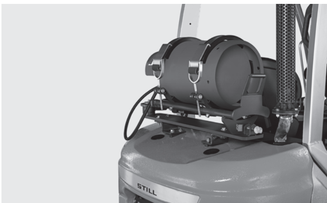
Changing gas cylinders is quick and easy thanks to the ergonomic cylinder holder with its swivel and fold-out mechanism, in normal working position here
