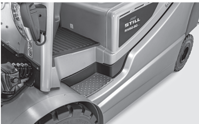
High level of safety thanks to large, non-slip steps for easy entry
