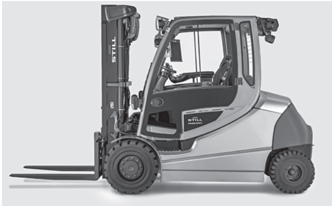
Full cab for outdoor use in all weathers
