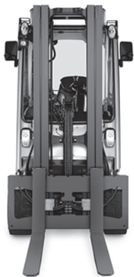
Slim mast ensures excellent view of the forks and extremely high safety standards
