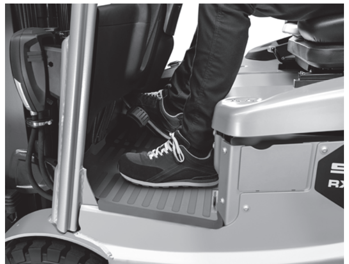
To provide an ergonomic workplace and comfortable access, the RXE has a spacious footwell despite its compact dimensions
